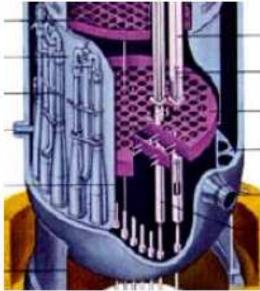
Jet Pumps & CRGT
