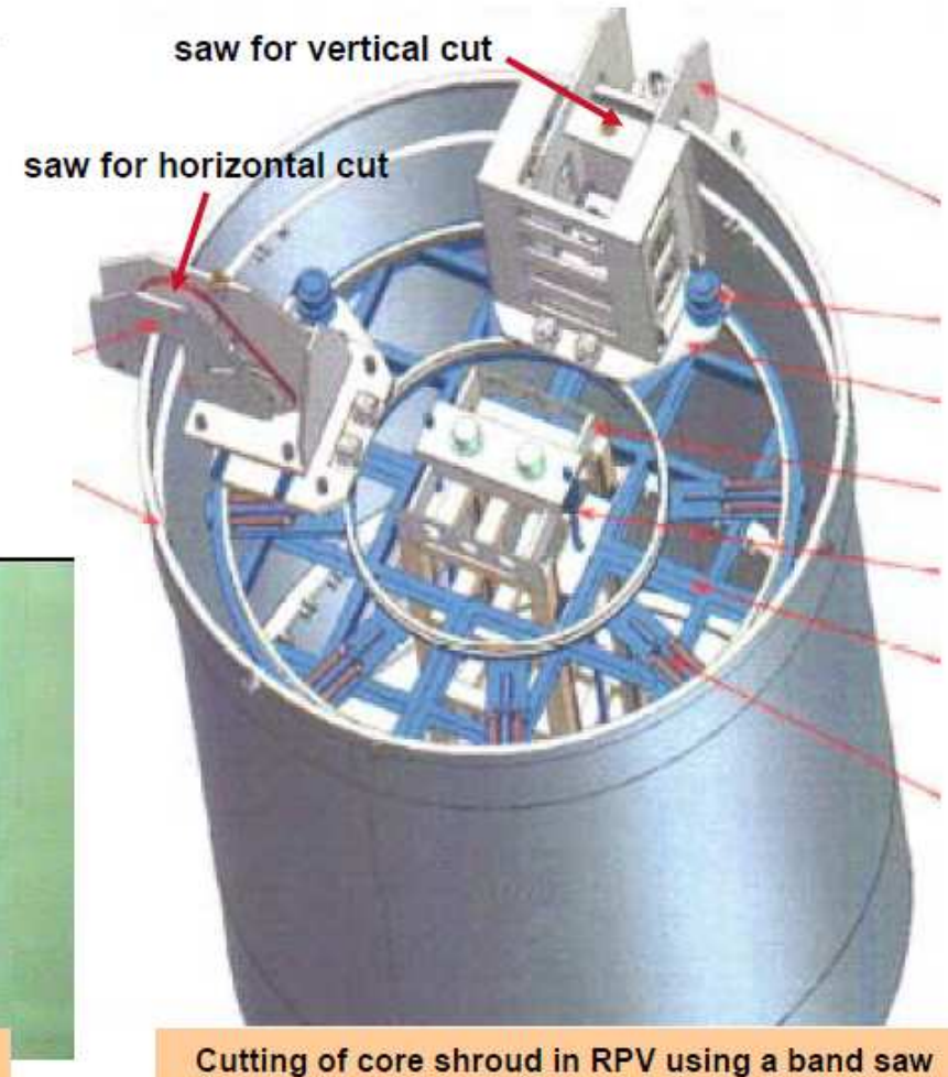
First cut on core shroud
